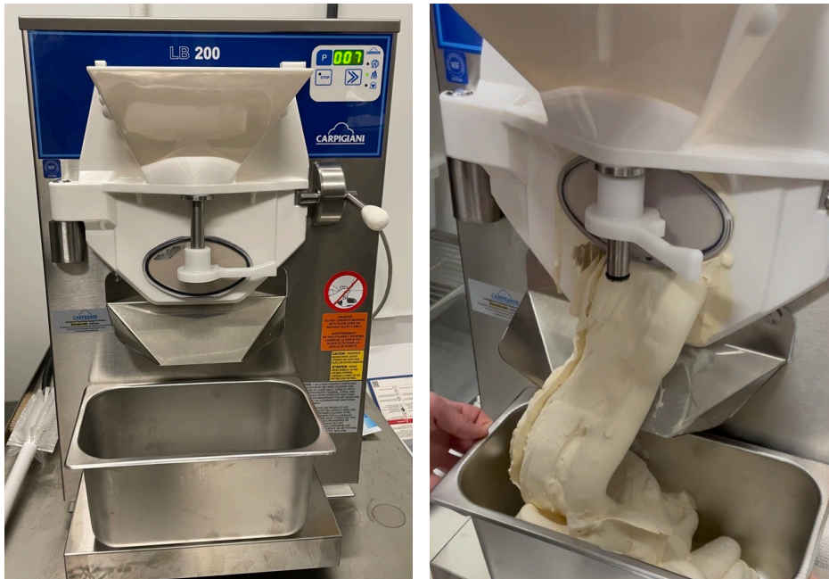
Fig. Batch freezer (Carpigiani, Bologna, Italy, LB 200 G up to 4.7 L)
